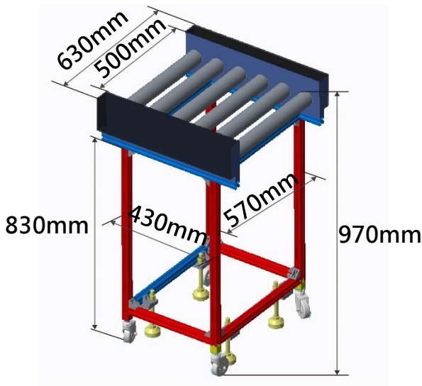
Figure 3: Roller Coaster (Unit: mm)
